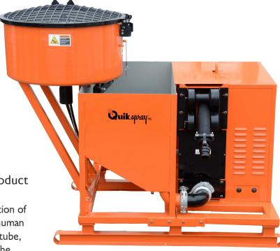
The parabolic hoppers are designed for easy flow of materials, and have no corners to clog. The specially designed 8-jet venturi spray nozzle for fiber filled coatings eliminates clogging. Cleaning is absurdly simple. A cellulose sponge is inserted in the bottom of the hopper, and pulled through by the pumping action with clean water.
