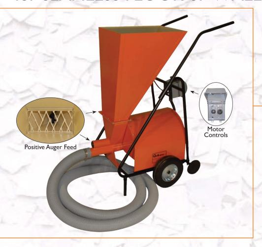
The Quikspray Commercial Chip Sprayer<sup>™</sup> features a 2-speed 2-3HP blower with 150/196 cfm of air with a velocity up to 33,570 fpm. The transfer and metering of the chip is accomplished with a positive, but variable speed auger feed powered by a separate gear reduced motor. The fast application of chips into wet resin eliminates a stop and go procedure. Both motors operate on 110VAC.
