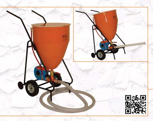
The Quikspray® AG-Blower will place quartz aggregate, sand, fillers, or non-skid granuals at a rate of 30-45 lbs/min into unset epoxy, cement, or polyester basecoats.
